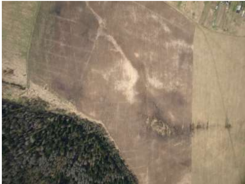
Figure 3. Fragment of the air picture of the malfunctioned underground drainage system.
